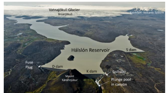
Figure 4. The Háslón reservoir, dams, spillway and fuse plug (Sigtryggdóttir et al., 2016). Photo: Emil Thor.
