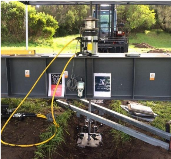
Figure 3. Pullout tests setup
