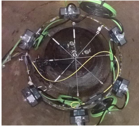
Figure 6 - Steel plate pre-equipped with Morphosense sensors and photo taken in micro-tunnel.
