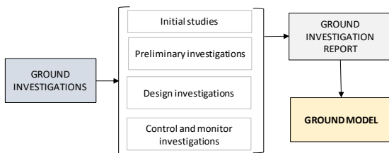
Figure 3. Ground modelling steps
