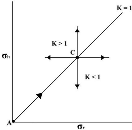
Figure 2. Variation of stress ratio  $K$  during saturation and consolidation. Point  $A$  corresponds to the state at the start of saturation while point  $C$  to the state at the start and end of consolidation.
