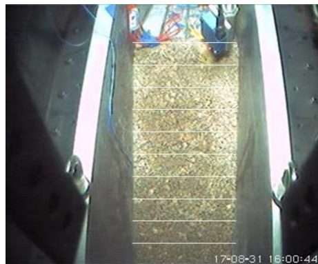
Figure 8. Pictures of the downstream slope taken (a) before and (b) after shaking in T3-0.36g.
