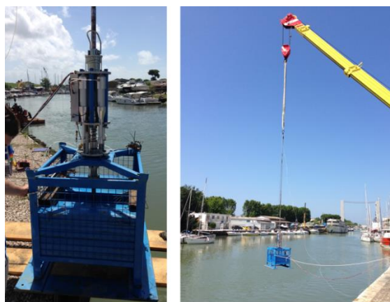
Figure 10. Seafloor DMT (Marchetti D. 2018)
