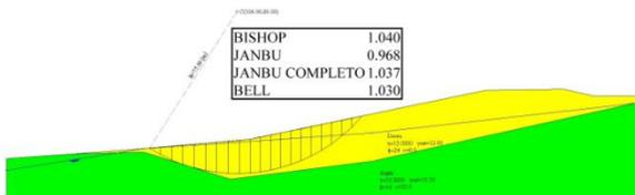
Figure 11. Case study – old landfill – LEM stability analyses static conditions, characteristic values  $F_s = 0.97$
