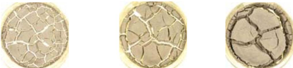
Figure 4: Crack pattern for 5, 10 & 20 mm thick specimens (left to right) at 75cm lamp distance
