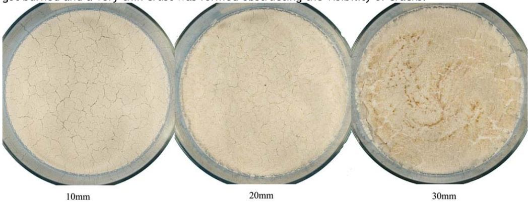
Figure 1: Crack pattern on potato starch for various specimen thicknesses (lamp distance = 50cm)
