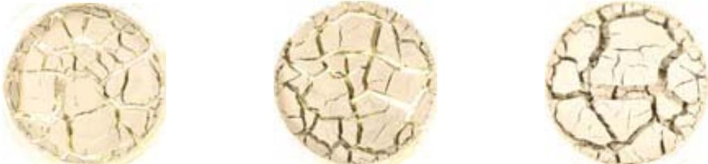
Figure 2: Crack pattern for 5, 10 & 20 mm thick specimens (left to right) at 35cm lamp distance
