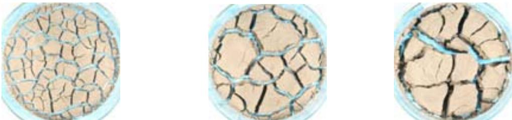
Figure 3: Crack pattern for 5, 10 & 20 mm thick specimens (left to right) at 50cm lamp distance
