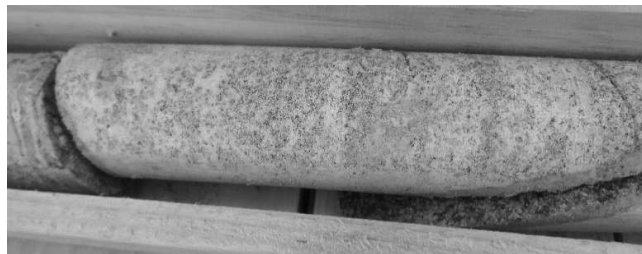
Figure 14. Portion of the residual norite core from 13.33 -14.02 m (BH1)
