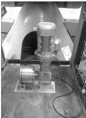
Figure 1. Model drum on the geotechnical centrifuge model platform
