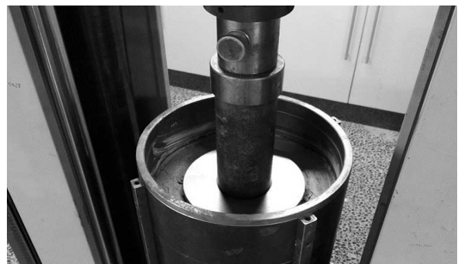
Figure 2. Test specimen at LL, with the loading plate and cylinder, prior to testing
