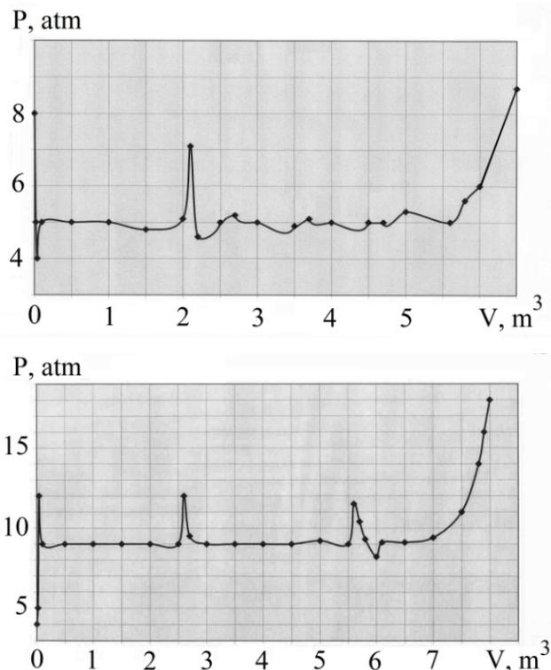
Figure 5. Typical dependences of the pressure on the volume of injection.
