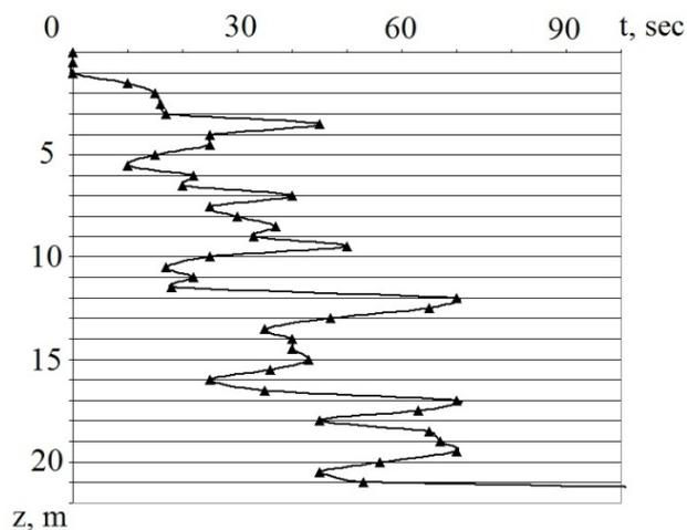
Figure 4. Schedule of a dynamic sounding of soils during the workflow (dependence of the injector sink rate on the density of the soil composition).
