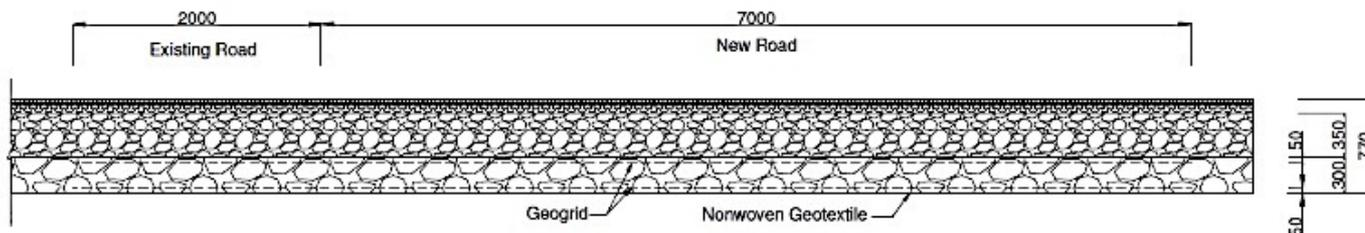
Figure 3. Standard cross section
