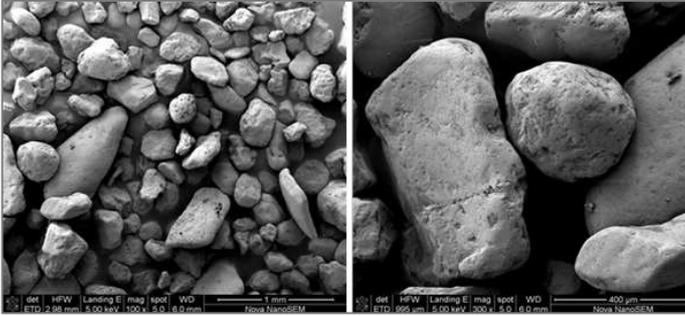
Figure 1. Cape Flats sand photomicrographs under 1 mm and 400  $\mu\text{m}$  levels of magnification
