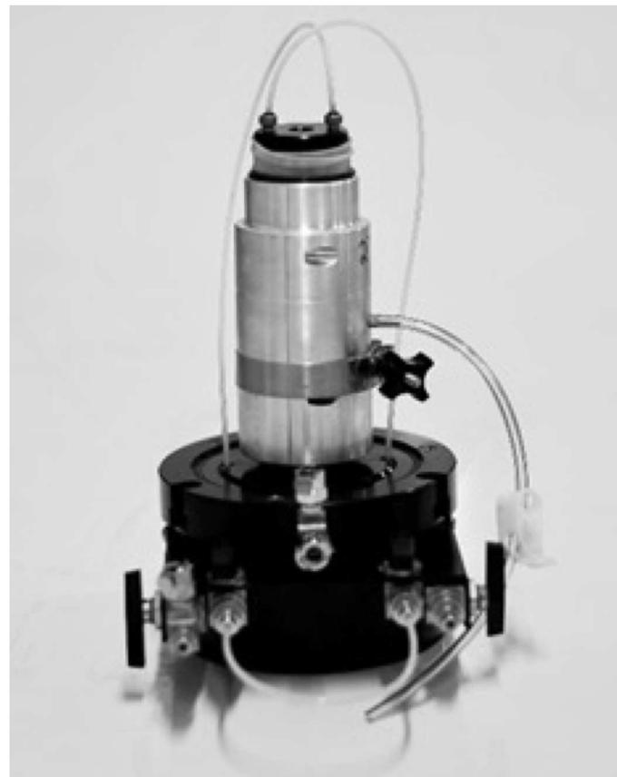
Figure 4. Specimen prepared in a split mould
