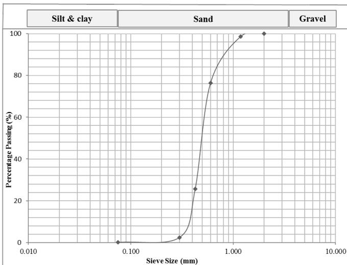
Figure 2. Grading curve for Cape Flats sand
