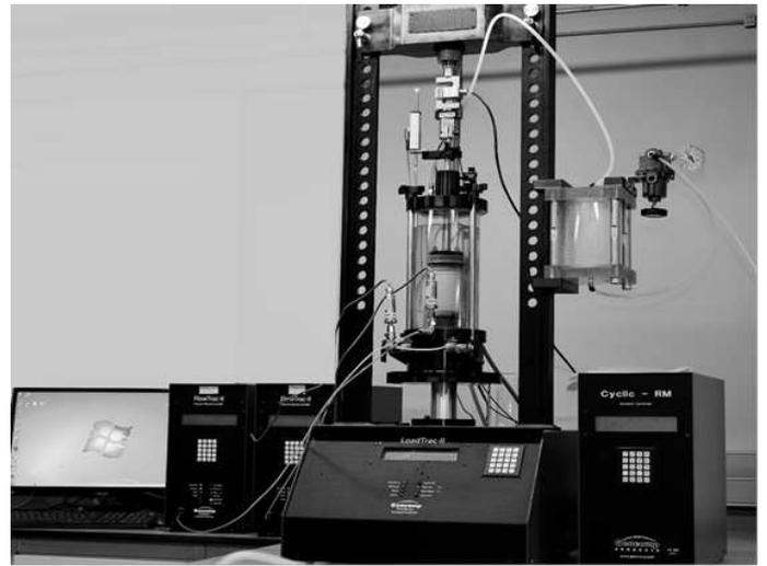
Figure 5. Test specimen in triaxial cell chamber mounted on platen ready for testing
