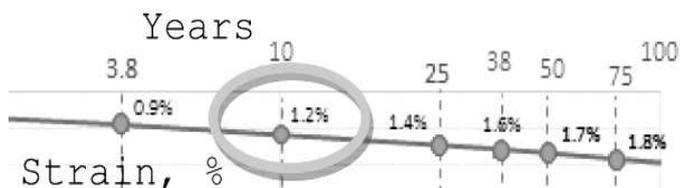
Figure 7. Creep curve and creep strain for the NPA geocells used (modified from PRS 2017)
