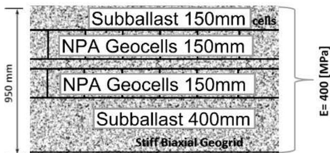
Figure 3. Geocell solution for the Nahariya railway (modified from Kief 2016)
