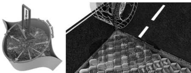
Figure 1. Illustration of geocell bearing mechanisms: single cell, left, and geocell system, right
