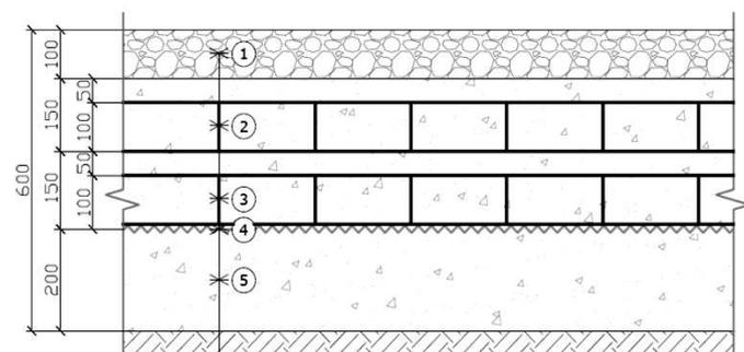
Figure 9. Cross-section of the final optimized solution with geocells for the Rubkona airfield (modified from PRS 2017)
