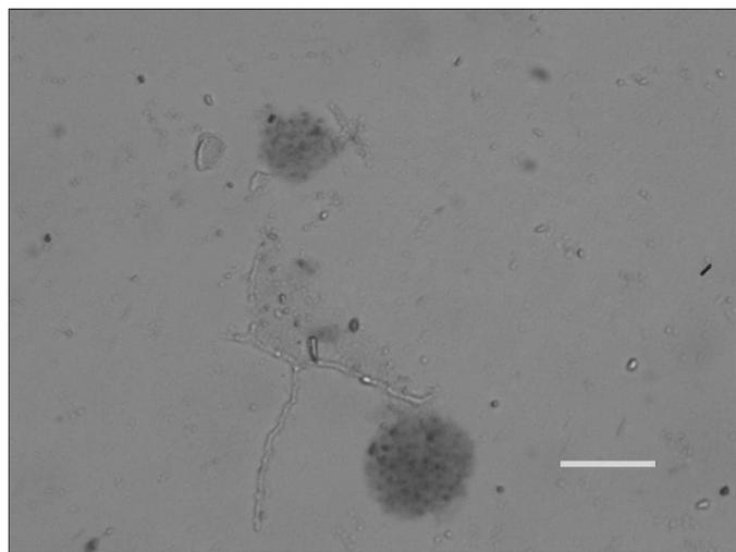
Figure 5. Medium-high magnification view (x40) of high-plasticity clay after the addition of  $3.25 \text{ g.dm}^{-3}$   $\text{Na}_2\text{S}_2\text{O}_8$ . The root hair at lower centre has no colloids surrounding it. Scale bar  $30\mu\text{m} \times 2\mu\text{m}$ .
