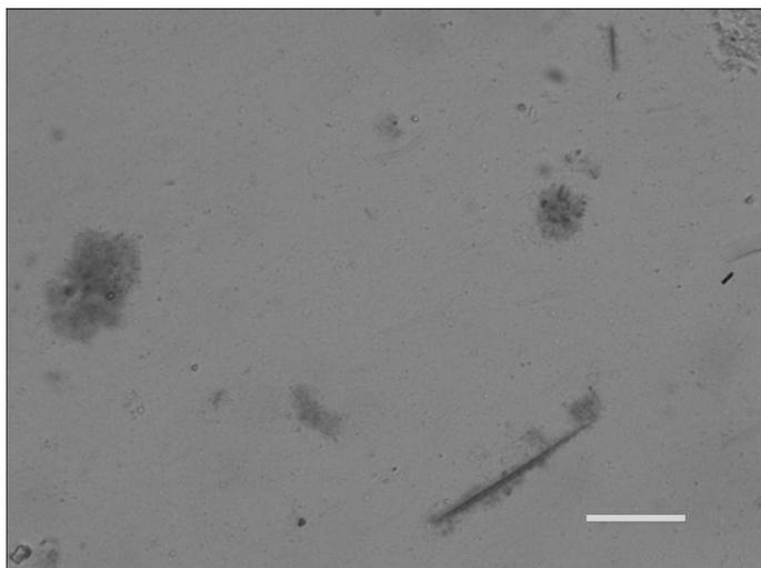
Figure 4. Medium-high magnification view (x40) of high-plasticity clay suspension without treatment. The root hairs at lower right and upper right are completely covered with colloids. Scale bar  $30\mu\text{m} \times 2\mu\text{m}$ .
