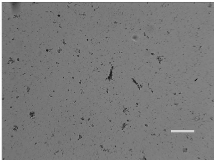
Figure 2. Low power view (x10) of compost suspension after the addition of  $3.7 \text{ g.dm}^{-3} \text{ Na}_2\text{S}_2\text{O}_8$  scale bar  $100 \mu\text{m} \times 10 \mu\text{m}$
