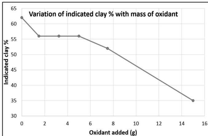
Figure 3. Indicated clay fraction for various quantities of  $\text{Na}_2\text{S}_2\text{O}_8$  added during preparation
