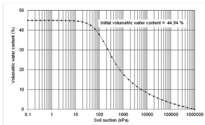
Figure 16. Volumetric water content,  $\theta$ , versus soil suction
