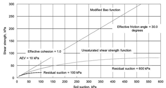
Figure 27. Effect of residual suction on the shape of the shear strength function
