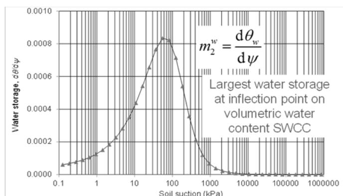
Figure 23. Water storage function for the artificial clayey silt soil.
