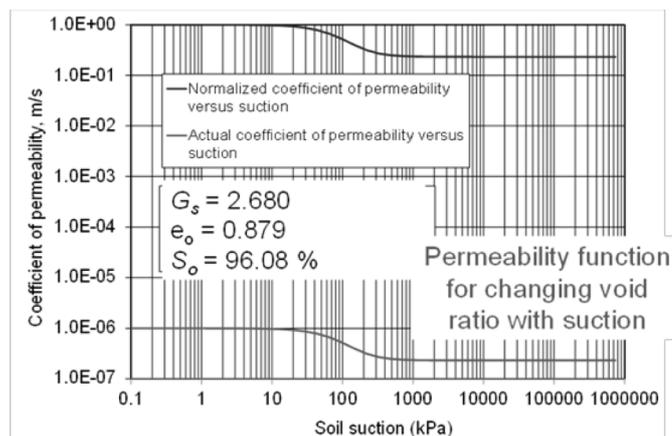
Figure 22. Changes in the permeability function in response to changes in void ratio.
