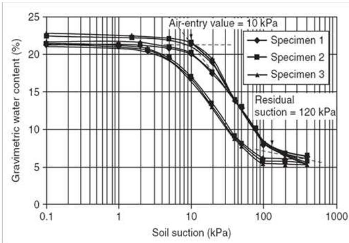
Figure 8. Drying and wetting SWCCs measured on a silt soil using the Pressure Plate apparatus (Pham, 2002)
