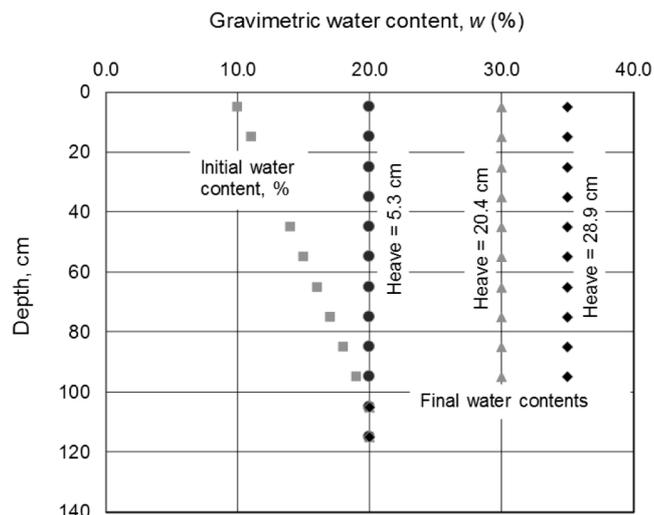
Figure 29. Prediction of heave calculations for 3 different assumed final water content conditions
