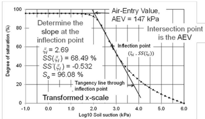
Figure 18. Definition of terms used on the substitution equation for the calculation of the “true” air-entry value.
