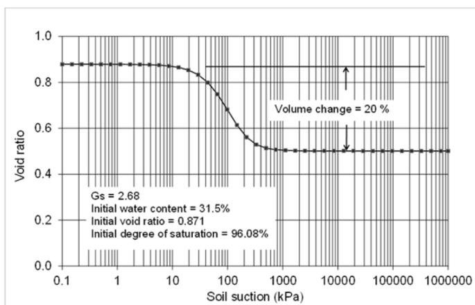
Figure 15. Void ratio versus soil suction showing volume change.
