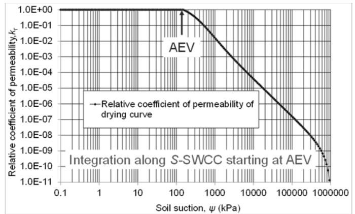
Figure 19. Relative permeability function for the artificial clayey silt as soil suction is increased beyond “true” air-entry value
