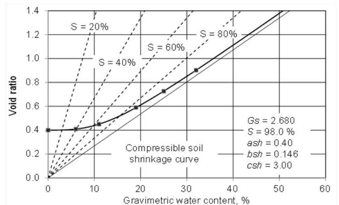
Figure 11. Typical shrinkage curve for a compressible soil.
