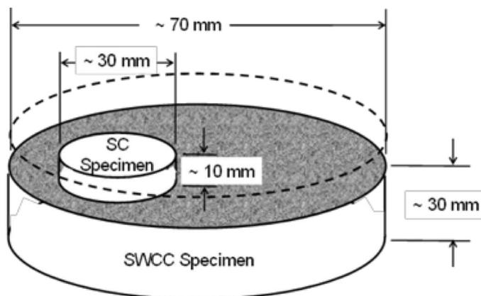
Figure 6. Use of similar initial volume-mass conditions for the  $w$ -SWCC and SC tests
