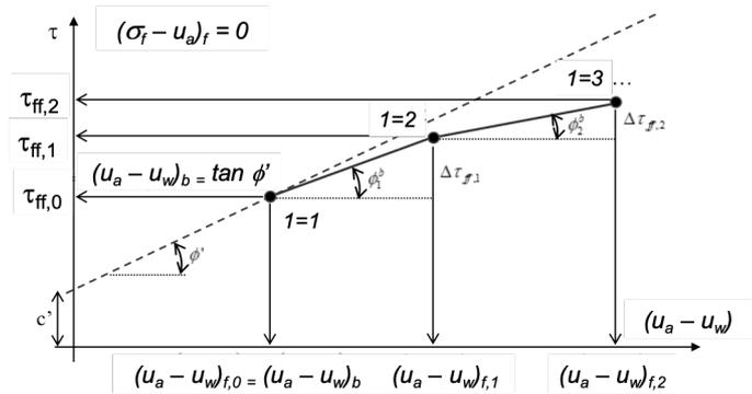
Figure 25. Marching forward process using the incremental tangent method
