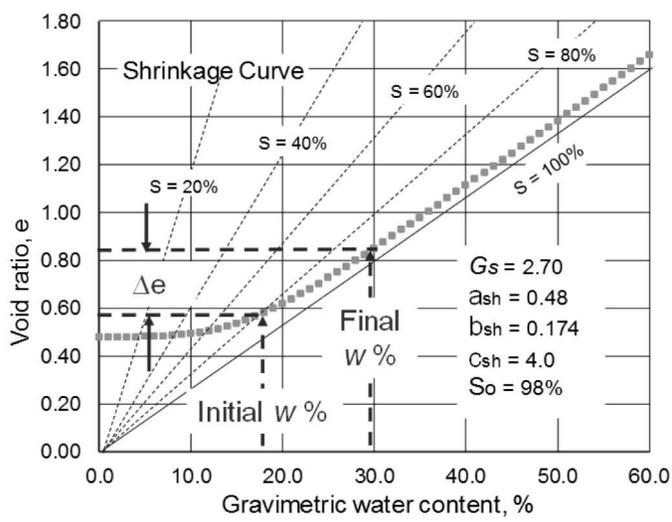
Figure 28. Shrinkage curve for the prediction of heave example
