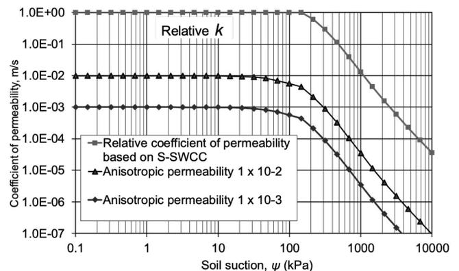
Figure 21. Scaling of the permeability functions for an anisotropic soil
