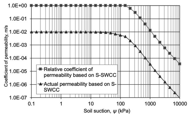
Figure 20. Scaling between the relative and actual permeability functions
