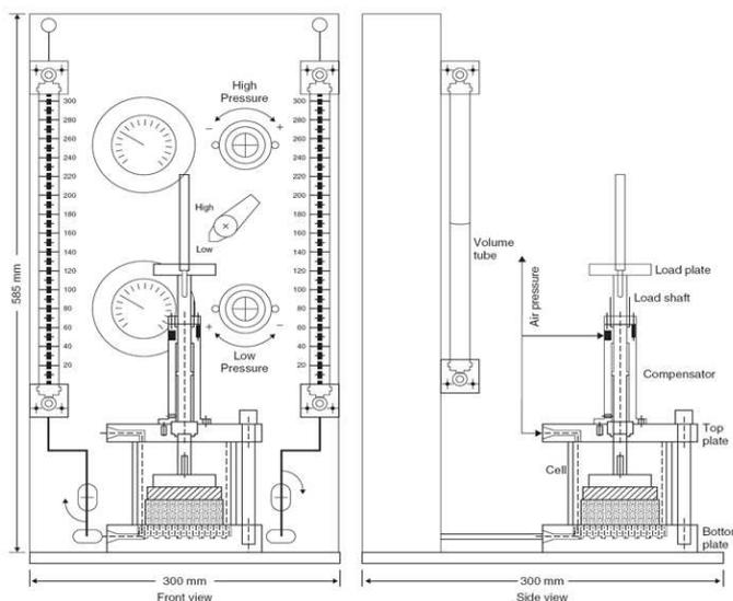
Figure 7. Front and side views of Pressure Plate cell (Courtesy of GCTS, AZ)
