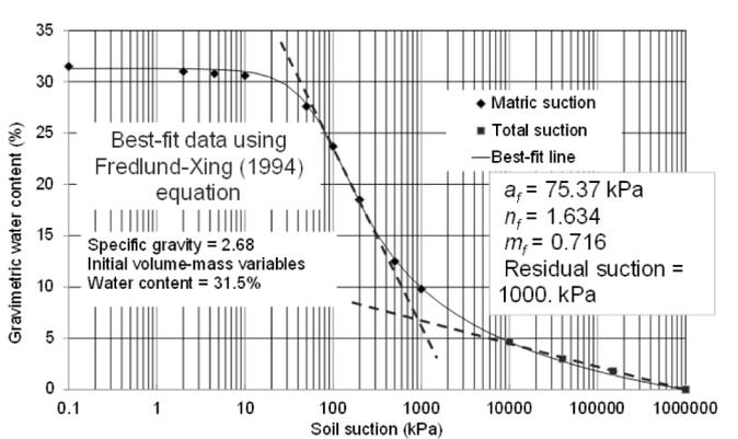
Figure 9. Soil suction data with best-fit Fredlund-Xing (1994) SWCC function for the artificial clayey silt
