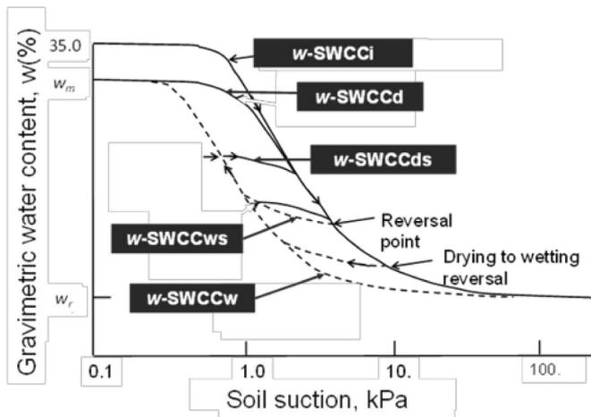
Figure 5. Suggested labelling for the gravimetric water content versus soil suction family of curves
