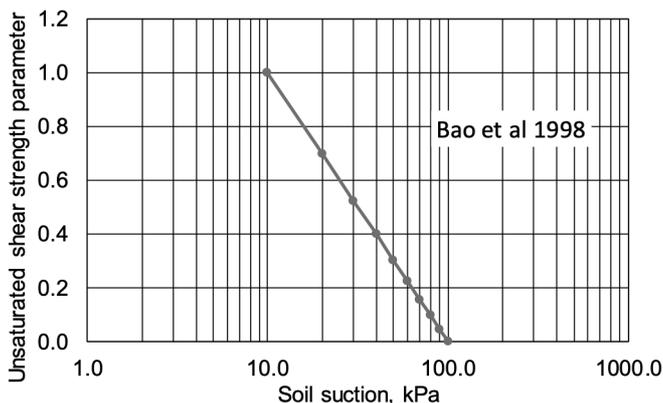
Figure 24. Proposed shear strength parameter by Bao et al., (1998) for an unsaturated soil
