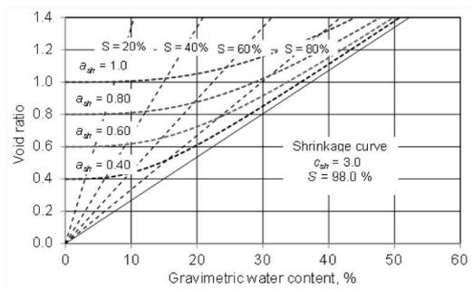
Figure 12. Effect of varying the ash fitting parameter of the shrinkage curve
