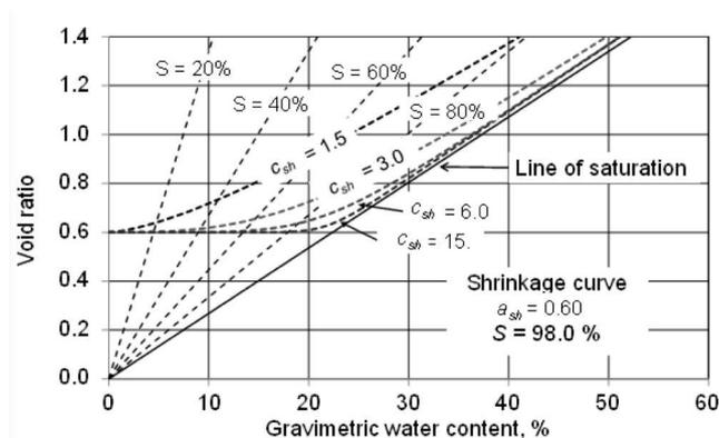
Figure 13. Effect of varying  $c_{sh}$  on the shrinkage curve
