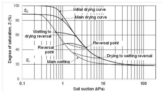
Figure 4. Hysteresis with respect to drying and wetting curves of degree of saturation versus soil suction for an unsaturated soil (modified from Klute 1986)
