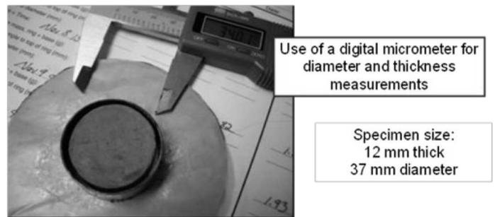
Figure 10. Measurement of the “Shrinkage Curve”, SC using micrometer calipers
