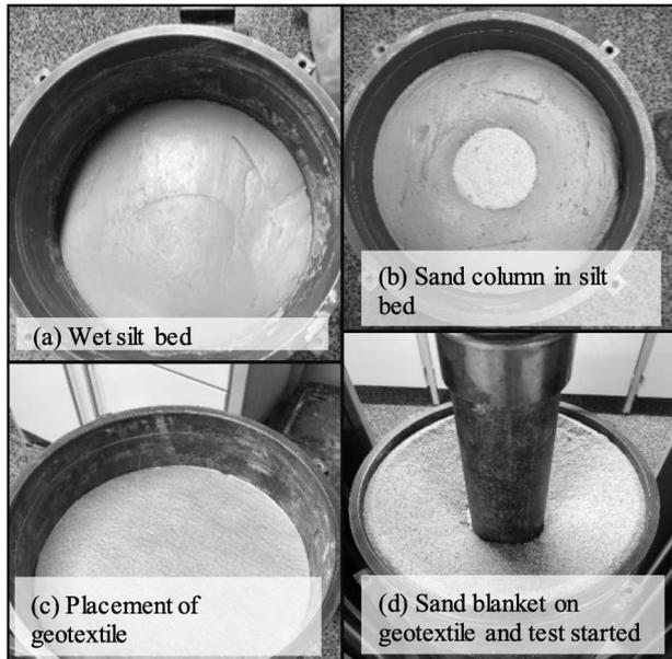
Figure 1. Test sample preparation and experimental set-up
