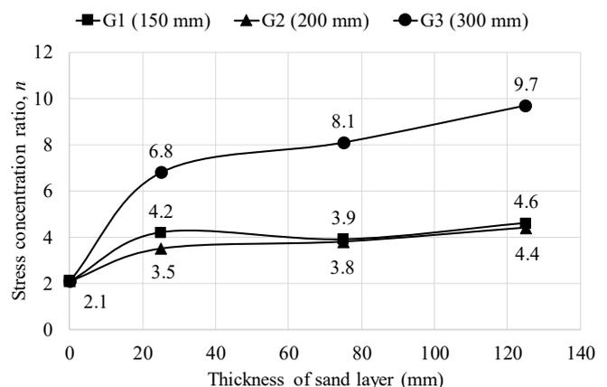
Figure 4. Stress concentration ratio determined for each test
