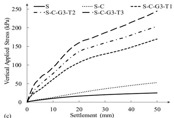
Figure 2. Stress-settlement characteristics for tests with geotextile diameters of a) 150 mm, b) 200 mm and c) 300 mm
