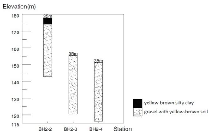
Figure 3. Boring Logs
