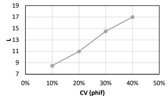
Figure 6. Variation of length strength with the CV ( $\varphi_f$ )
