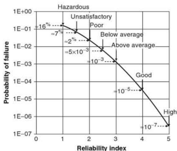
Figure 2. Probability of failure vs reliability index (from US Army Corps of Engineers 1997)
