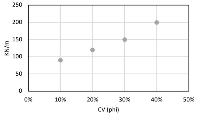
Figure 4. Variation of tensile strength with the CV ( $\varphi_b$ )
