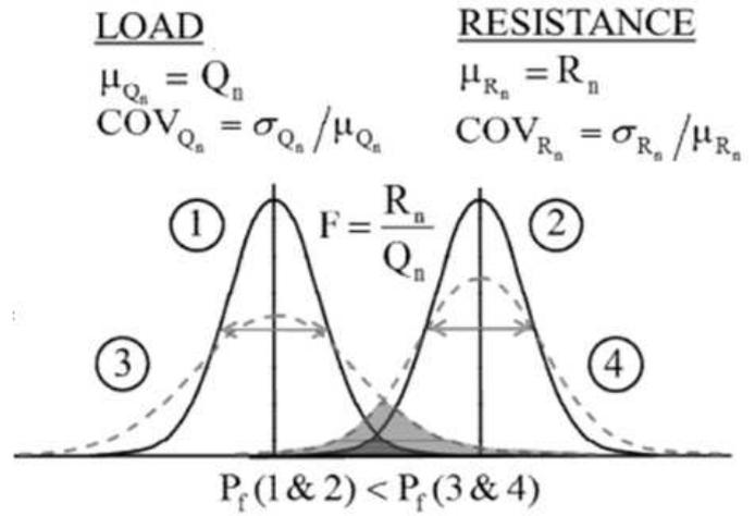
Figure 1b) Factor of safety and probability of failure concepts (modified from Bathurst 2018)
