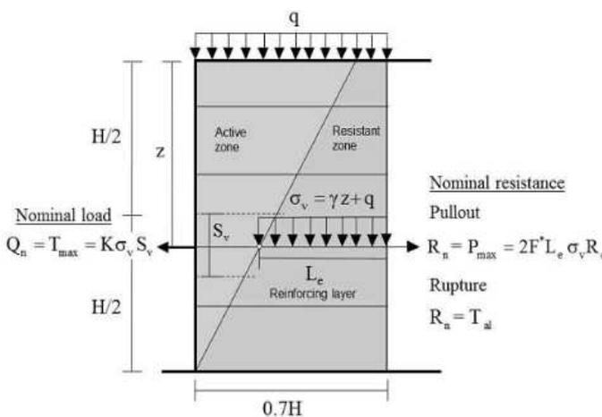
Figure 1a) Nominal load and resistance equations for reinforcement rupture and pull-out limit states for internal stability of GRSW (modified from Bathurst 2018)
