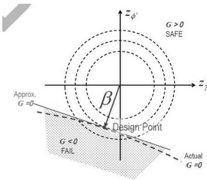
Figure 2: Illustration of the first order reliability method
