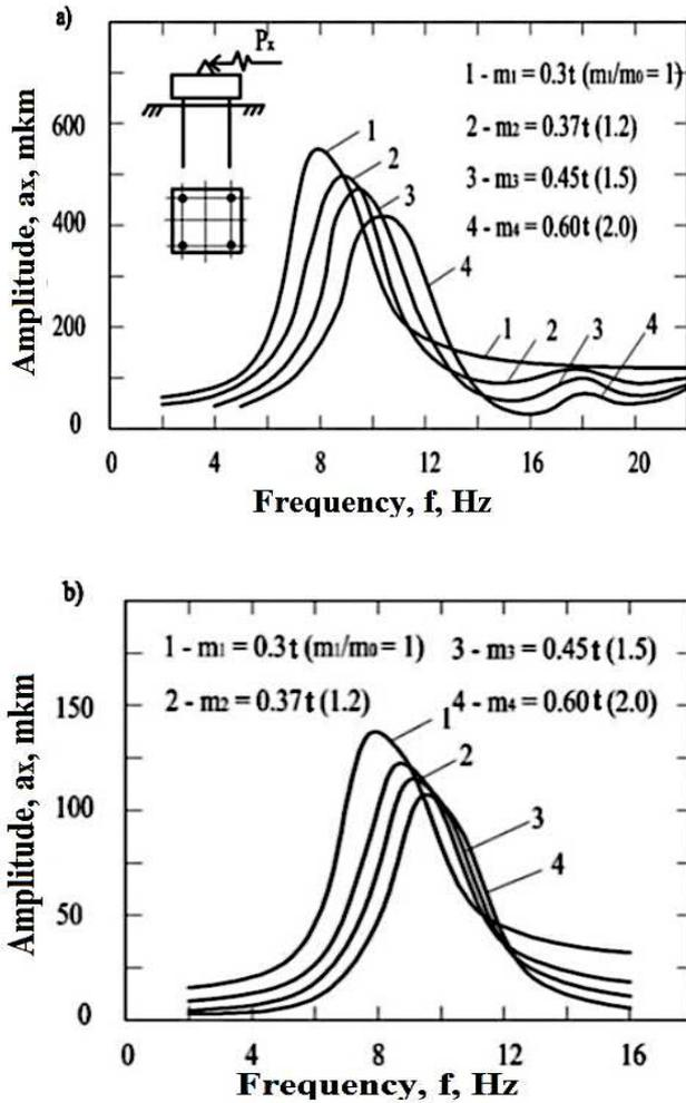
Figure 7. Flow diagrams of horizontal oscillations of pile foundation with foundation frameworks of various mass under experimental data (a) and numerical simulation results (b).
