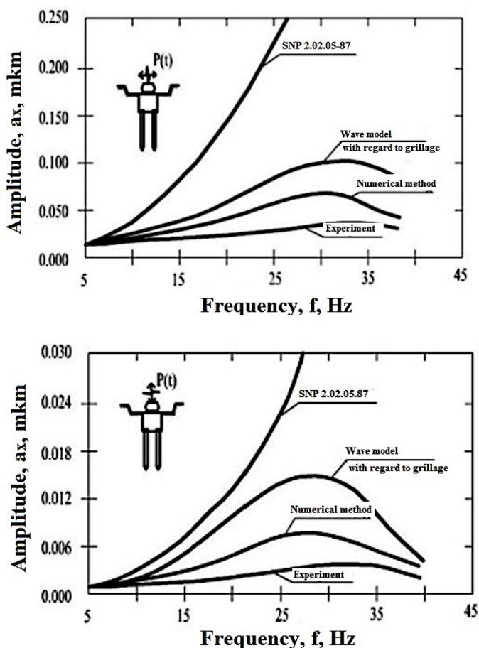
Figure 12. Flow diagrams of vertical (a) and horizontal (b) oscillations of a pile foundation with a ingrounded foundation framework, obtained experimentally (4), by a numerical method in SolidWorks package (3), calculated by the wave model (2) and by SP 26.13330.2012 (SNiP 2.02.05-87) (1).
