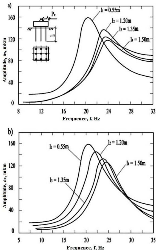
Figure 2. Flow diagrams of horizontal oscillations of pile foundation models with piles of various lengths under experimental data (a) and numerical simulation results (b).
