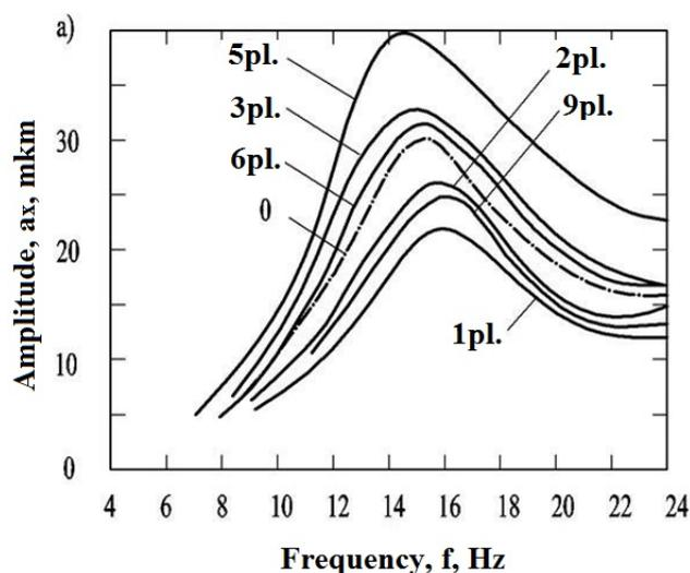
Figure 5. Flow diagrams of horizontal vibrations of pile foundations with different number of piles in the foundation framework according to experimental data.
