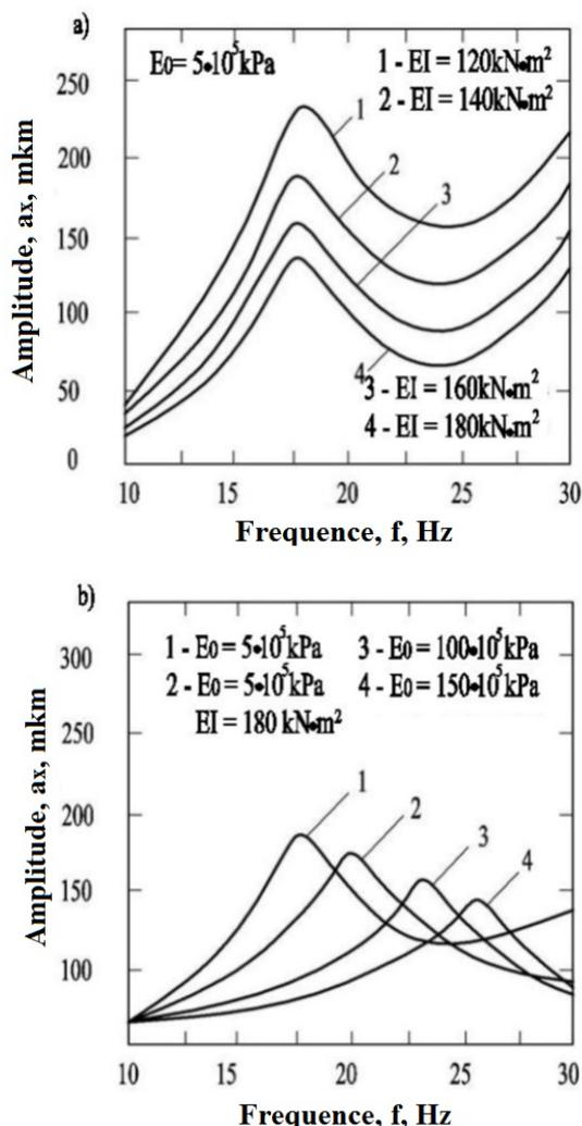
Figure 4. The effect of flexural rigidity of the pile (a) and the modulus of elasticity of the soil (b) on the parameters of the horizontal vibrations of the pile foundation according to the data of numerical simulation in the software package SolidWorks.
