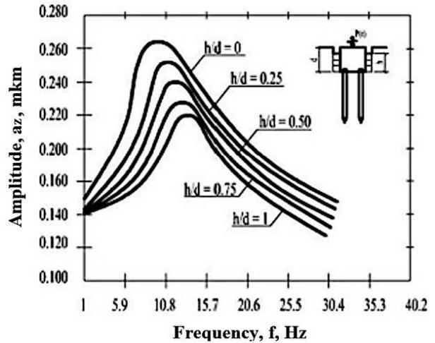
Figure 8. Flow diagrams of vertical oscillations of a pile foundation with an in ground foundation framework when changing the contact area of its side surfaces with the ground.
