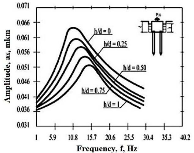
Figure 9. Flow diagrams of horizontal oscillations of a pile foundation with an in ground foundation framework when changing the contact area of its side surfaces with the ground.
