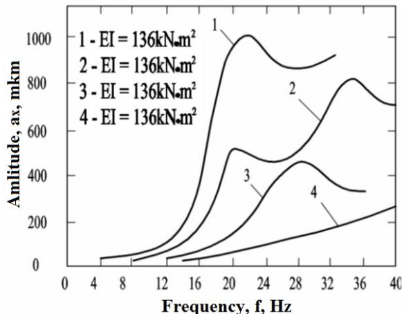
Figure 3. Flow diagrams of horizontal oscillations of the tested pile foundation with different flexural rigidity of piles and with a change in the modulus of elasticity of the soil 1, 2 - at  $E_0 = 3.8 \cdot 10^5$  kPa; 3 - at  $E_{01} = 3.8 \cdot 10^5$  kPa (up to 8d),  $E_{02} = 164.6 \cdot 10^5$  kPa (from 8d to 21d); 4 - at  $E_0 = 164.6 \cdot 10^5$  kPa (up to 20d).
