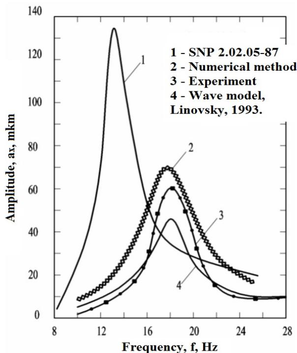
Figure 11. Amplitude-frequency flow diagrams of horizontal oscillations of a production pile foundation, obtained experimentally (3), by a numerical method in the SolidWorks package (2), calculated by the Linovsky wave model (4) and by SP 26.13330.2012 (SNiP 2.02.05-87) (1).
