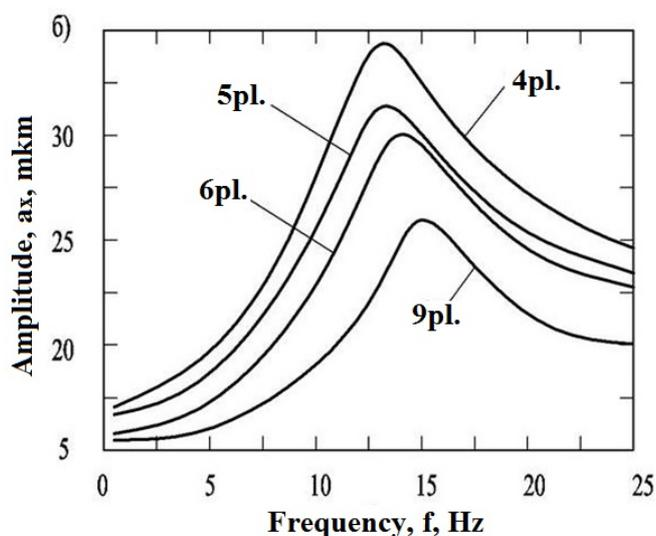
Figure 6. Flow diagrams of horizontal vibrations of pile foundations with different number of piles in the foundation framework according to the results of numerical modelling (b).
