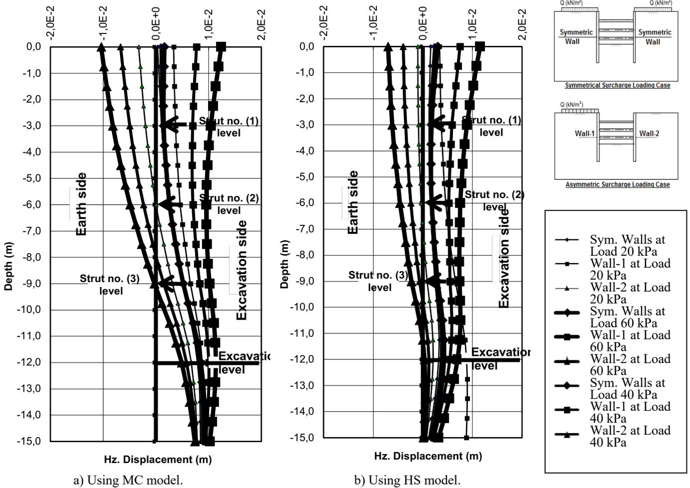
Figure 3. Horizontal displacement for model M2 at different values of symmetric and asymmetric surcharge loading.
