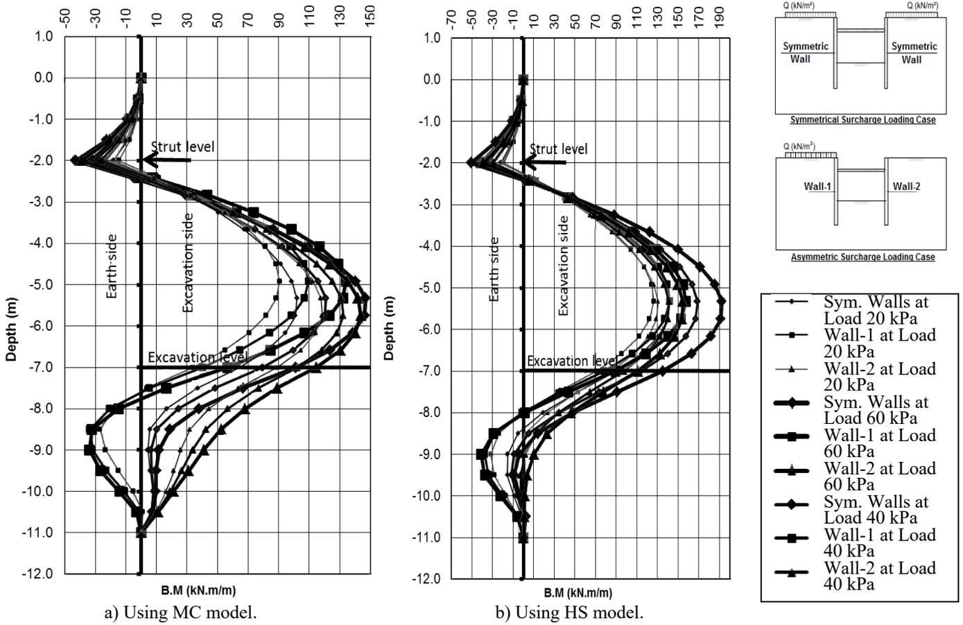
Figure 4. Bending Moment diagrams for model M1 at different values of symmetric and asymmetric surcharge loading
