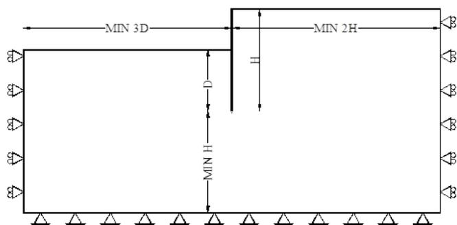
Figure 1. Minimum requirements for deep excavation problems (K.J. Bakker)
