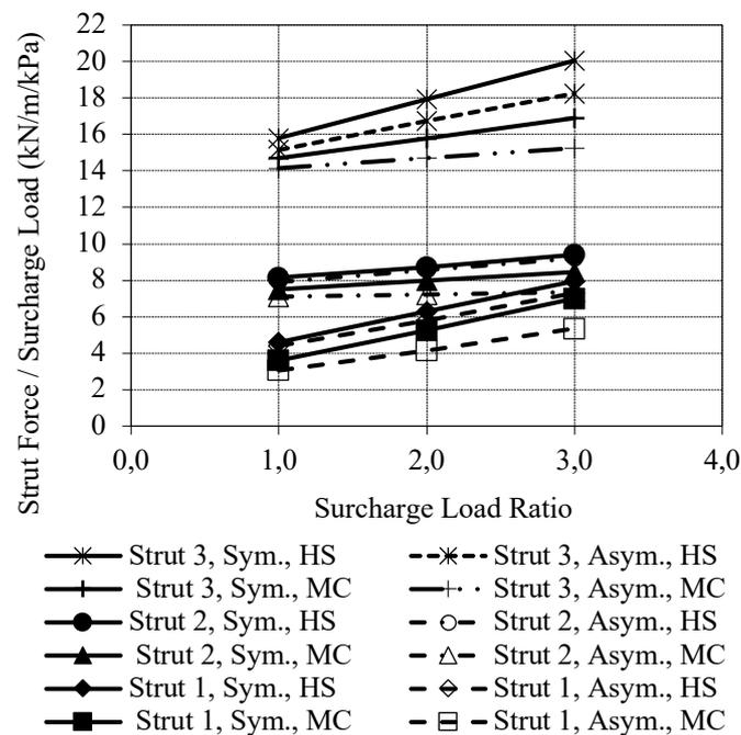
Figure 7. Strut force / Surcharge load vs Surcharge load ratio for model M2
