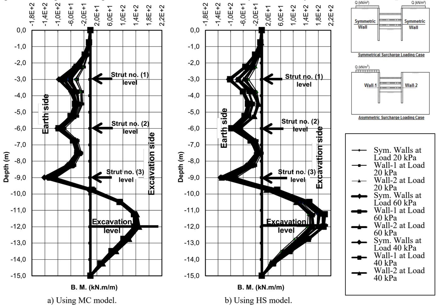
Figure 5. Bending Moment diagrams for model M2 at different values of symmetric and asymmetric surcharge loading
