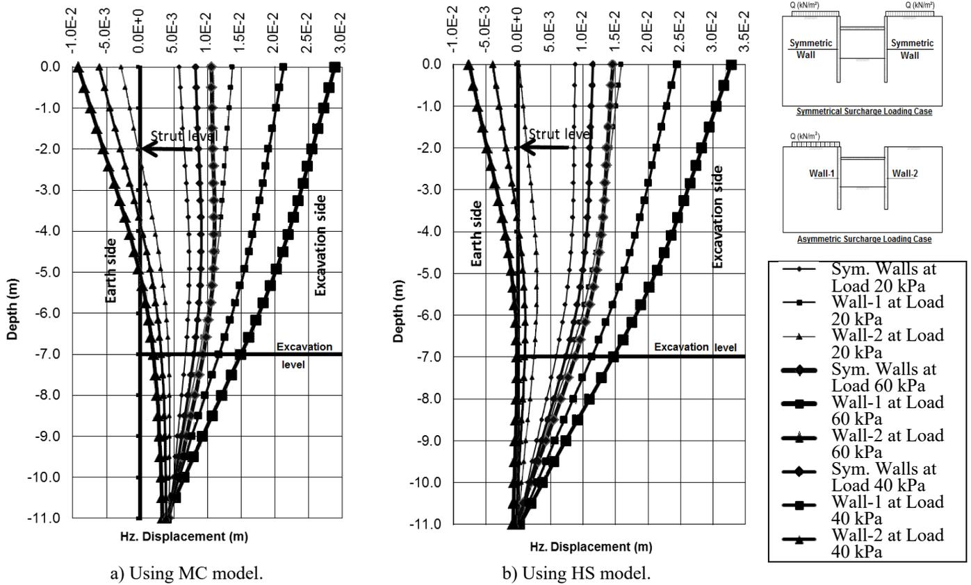
Figure 2. Horizontal displacement for model M1 at different values of symmetric and asymmetric surcharge loading.
