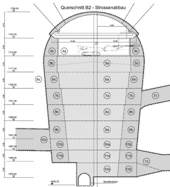
Figure 7. Cross-section of machine cavern with excavation stages and uppermost extensometers
