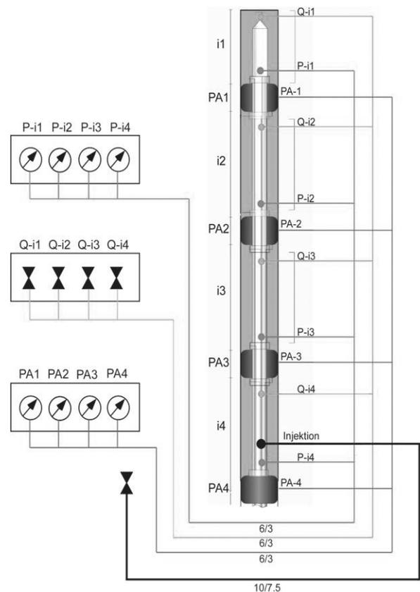
Figure 4. 4-fold packer system used for hydraulic testing
