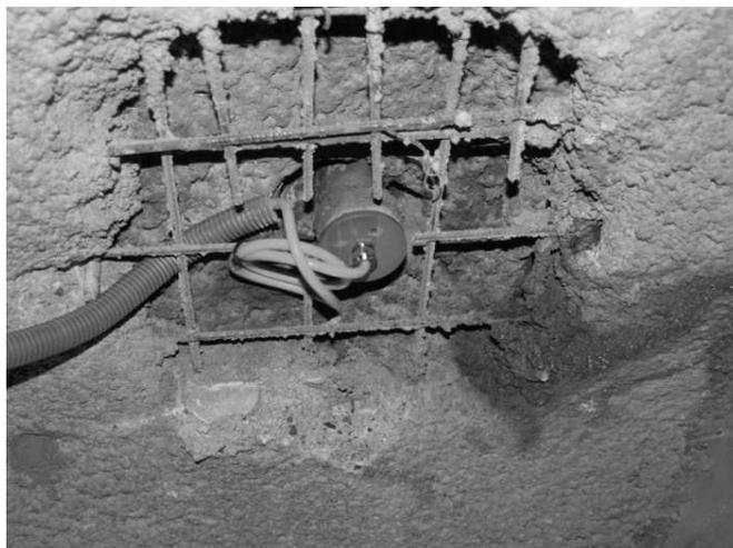
Figure 8. Extensometer head with bus cable
