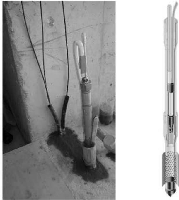
Figure 10. Piezopress: Installation with retrievable pressure sensor (left) and schematic cross-section (right)
