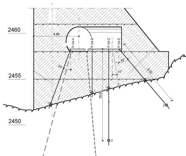
Figure 9. Measuring sections in the lake Mutt dam, dark solid lines represent the flotation measurement boreholes
