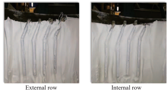
Fig. 5. Failure mechanism uncovered post-test.
