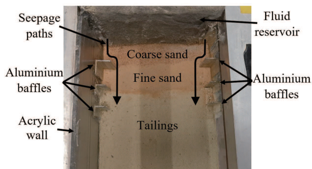
Fig. 5: Upstream view of model slope with aluminium baffles, sand filters and acrylic wall.
