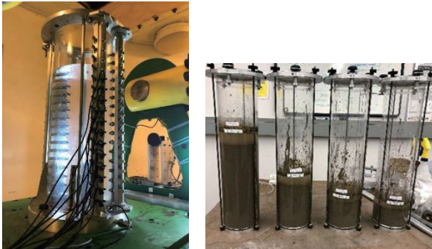
Fig. 1. Left: Consolidation cell with attached pore pressure transducers. Right: Tailings dispensers with tailing lift
