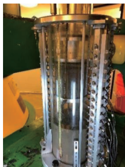
Fig.2. Depositing a new lift into the consolidation cell with the dispenser
