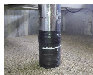
Fig. 1. a) overall configuration of test 2. b) local scouring of test 2. c) global scouring of test 3.
