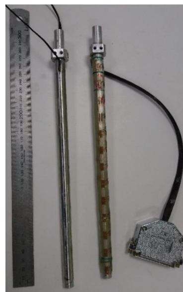
Fig. 2. Aluminium piles of same dimensions instrumented with optic fibre (left) and strain gauges (right).
