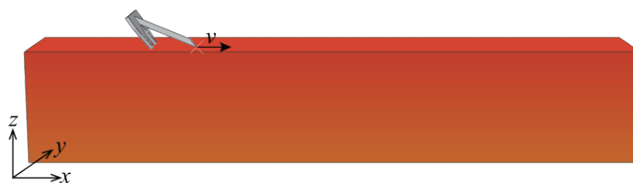
Fig. 7: Qualitative horizontal stress distribution for the embedding process of the DEA in sand: initial situation.
