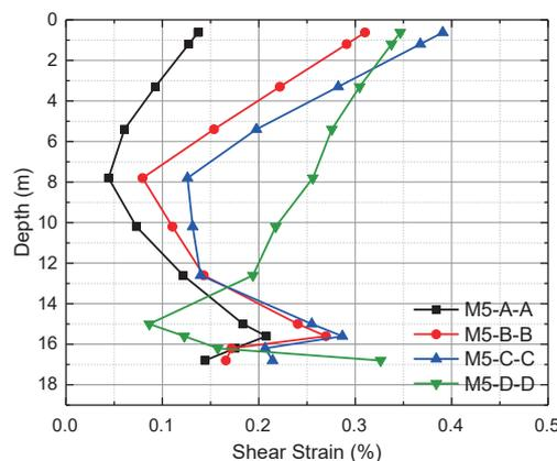
Fig. 3. Peak shear strains of the enclosed soil
