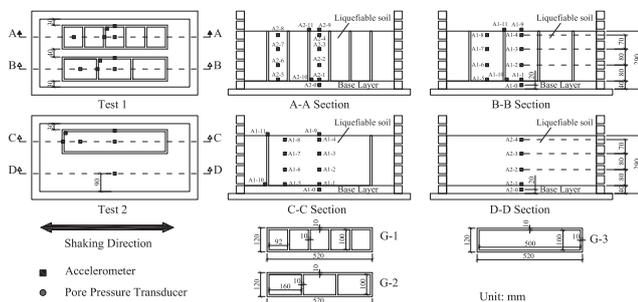
Fig. 1. Model configurations.
