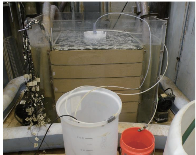
Fig. 1. Large-scale soil box.
