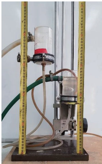
Fig. 1. The testing stand used for the investigation of the static liquefaction phenomenon.
