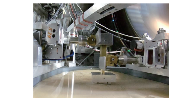
Fig. 6. Illustration and photo of the experimental setup for the pushover and combined loading tests.
