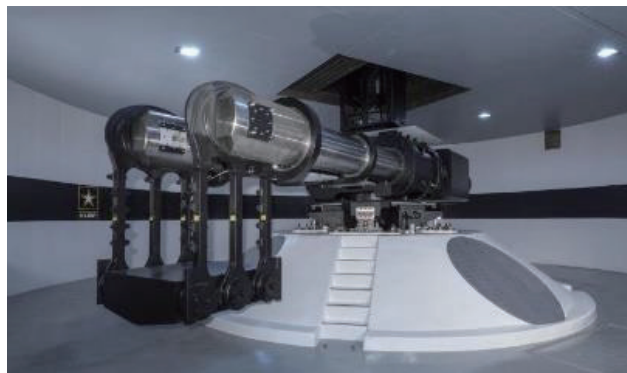
Fig 1. 1,200 g-ton, 6.5m radius centrifuge at ERDC after renovations. Aerodynamic shrouds not pictured.
