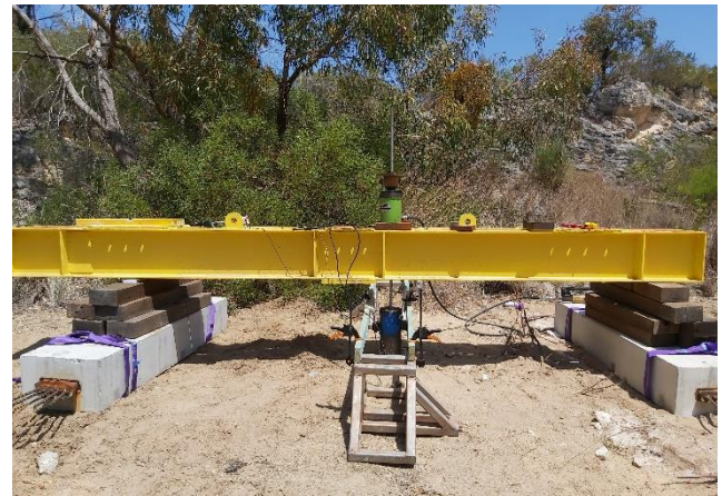
Figure 4. Pile capacity testing in variably cemented carbonate sand.
