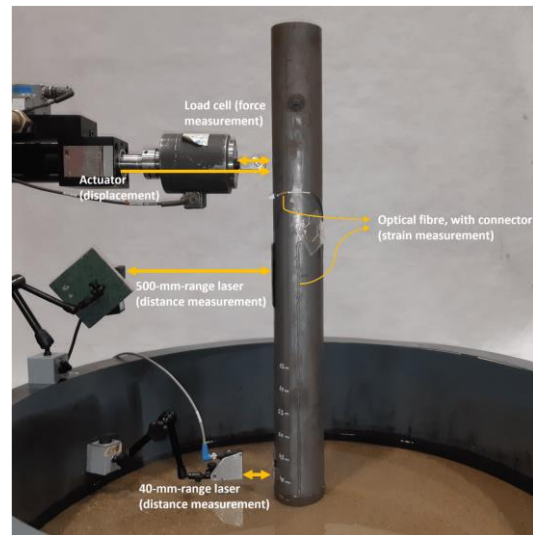
Figure 4 Pile setup for lateral loading
