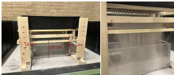
Figure 4 – Pluviometer and sample preparation
