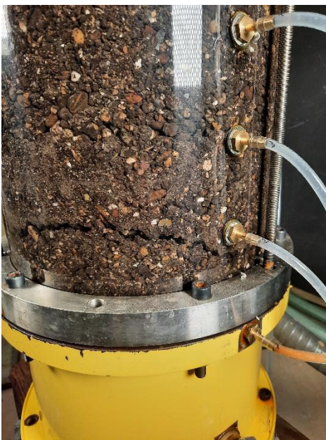
Figure 5. The 14% sand sample after the cyclic loading phase with fissure at the left part of the sample. Visible are the left side standpipe ports.
