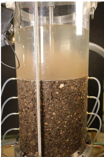
Figure 8. The disintegrated 6% sand sample at the end of testing at a head difference of 80 cm.
