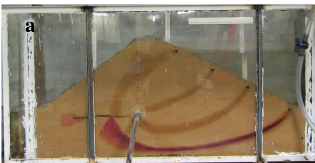
Figure 9. Physical model (a) and a numerical model (b) of an embankment with a horizontal, vertical filter and a relief drain.
