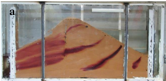
Figure 7. Physical model (a) and a numerical model (b) of an embankment with a vertical filter (no relief drain).
