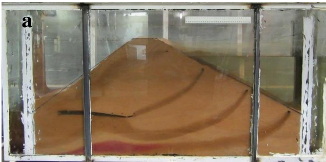
Figure 6. Physical model (a) and a numerical model (b) of an embankment with a horizontal filter (no relief drain).
