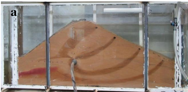
Figure 8. Physical model (a) and a numerical model (b) of an embankment with a vertical filter and a relief drain.
