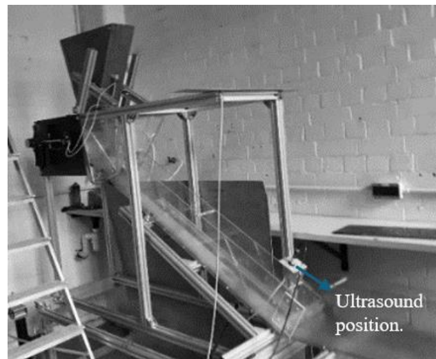
Figure 2. Flume apparatus photograph & diagram of slit barrier channel location.
