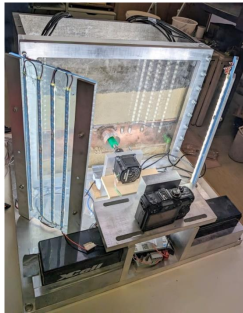
Figure 3. Model container with the required instrumentation ready to be placed in the centrifuge.
