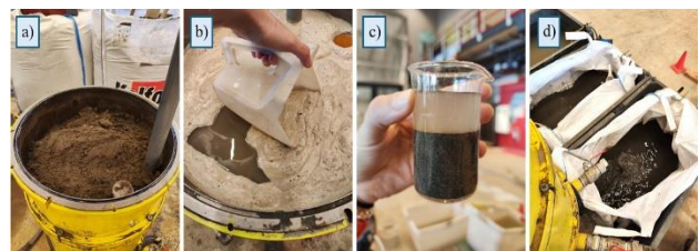
Figure 3. Soil preparation process: removal of fines.
