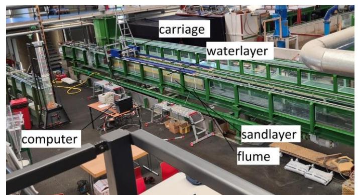
Figure 2. Water flume facility at TU Delft adapted for beam trawl gear experiment.
