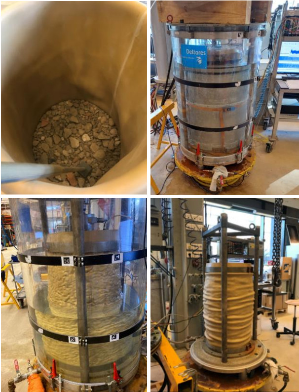
Figure 3. 0.45 m diameter drained triaxial tests on the fill
