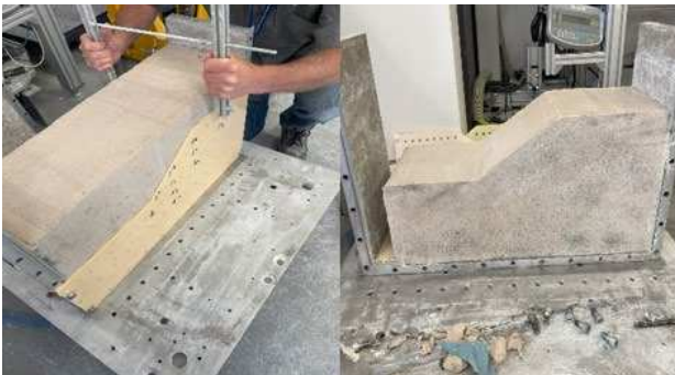
Figure 2-2 Model construction – left: template positioned before cutting compacted slope; right: slope after cutting.
