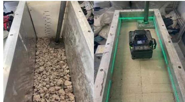
Figure 2-1 Soil preparation and compaction.
