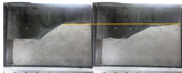
Figure 3-7 Crest settlement during auto balance phase.
