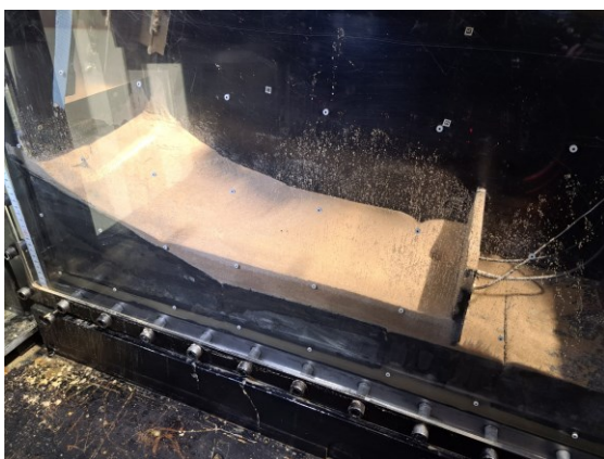
Figure 4. View of the centrifuge model at the end of a trial test with uniform sand.
