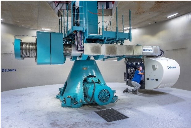
Figure 1. View of the GeoCentrifuge of Deltares, Netherlands (image courtesy of Deltares).
