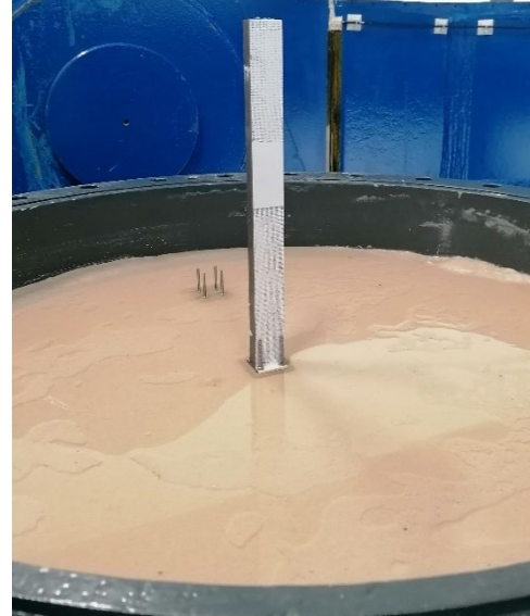
Figure 3: Catenary mast placed on top of the foundation.
