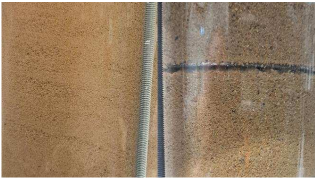
Figure 2: Separation of grains in the silo (left) and mixed sample over sieve (right)
