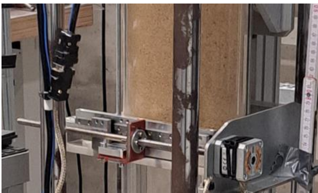
Figure 5: Rusting of the sand pluviation test stand
