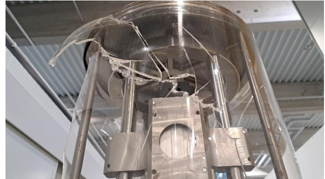
Figure 6: Failure of the original vacuum bell
